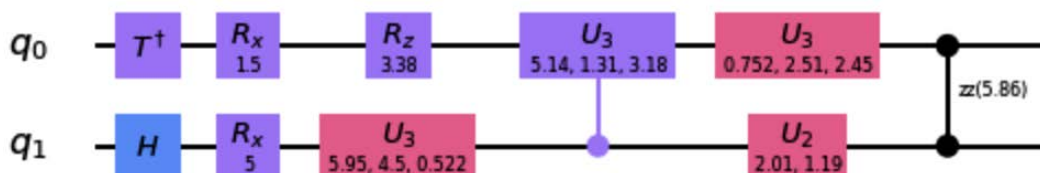
Figure 8.7 – Randomly generated two-qubit circuits with a depth of 6
