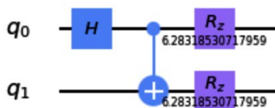
Figure 8.14 – Rotation gates R_z now have the Parameter value \theta set to 2\pi
